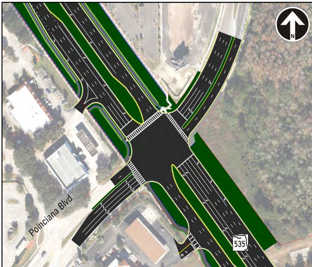
Figure 1-3 SR 535 and Poinciana Blvd Signalized Intersection Alternative
