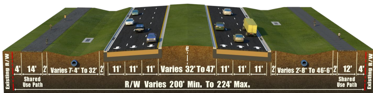
Figure 1-2: Preferred Alternative Typical Section
