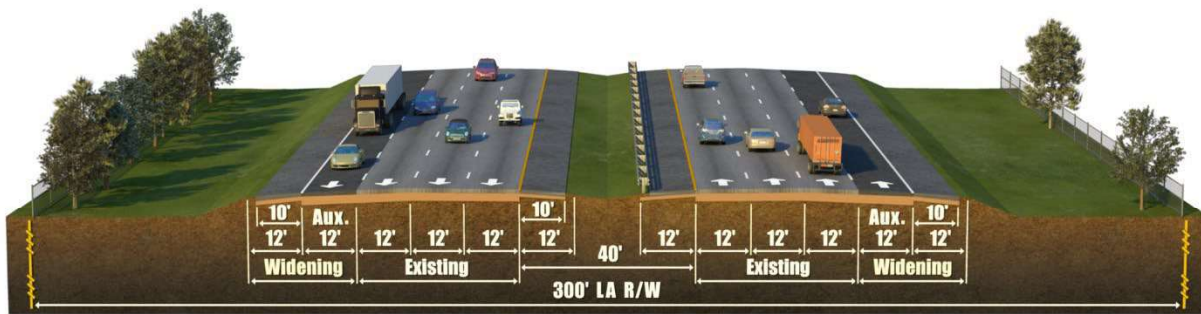
Figure 1-2: I-75 Preferred Alternative Typical Section
