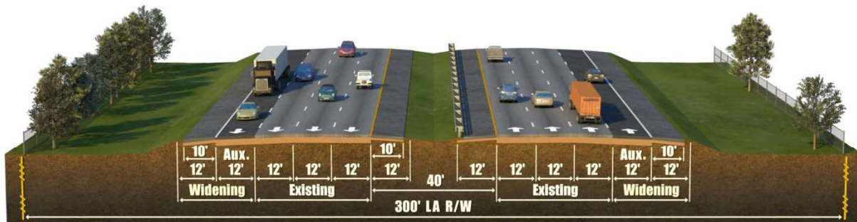
Figure 7-1: I-75 Proposed Typical Section
