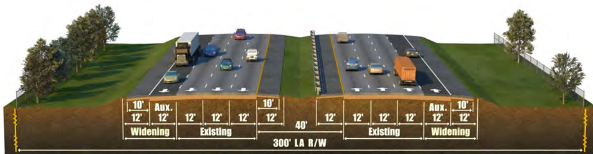
Figure 1-2 | Auxiliary Lanes Alternative Typical Section
