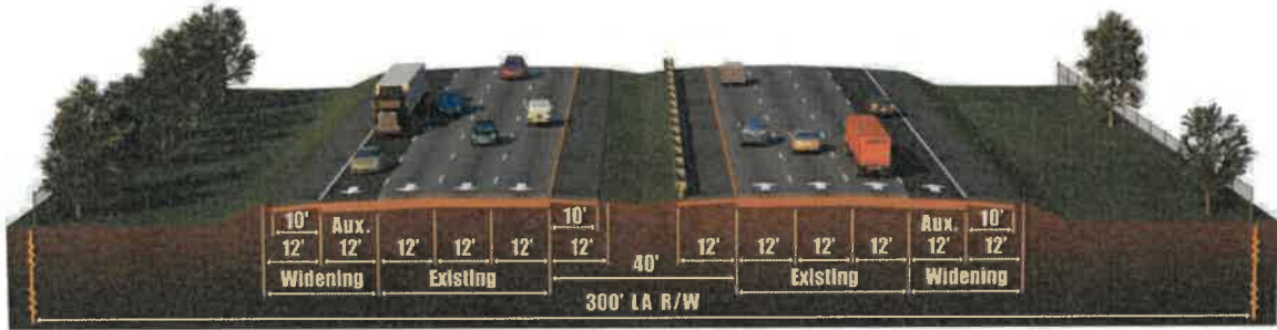
Figure 3: I-75 Typical Section
