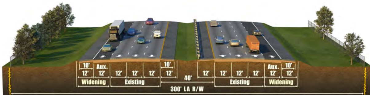
Figure 1-2 | Auxiliary Lanes Alternative Typical Section
