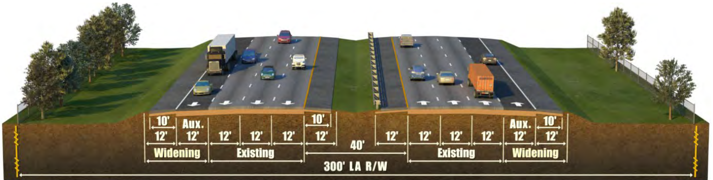
Figure 2.1: I-75 Auxiliary Lanes Alternative Typical Section
