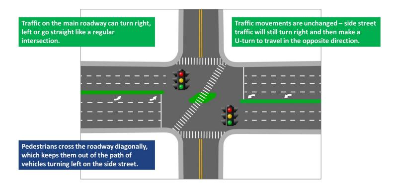
Above is an illustration of a signalized directional median opening. This is the type of crossing proposed at Chicory Lane. For this type of crossing, traffic on S.R. 436 will have a continuous green light until a pedestrian activates the signal to cross. The light will then change from green to yellow and then to red, and the pedestrian will be given the Walk signal to cross. This type of crossing helps to reduce pedestrian conflicts with turning vehicles.
