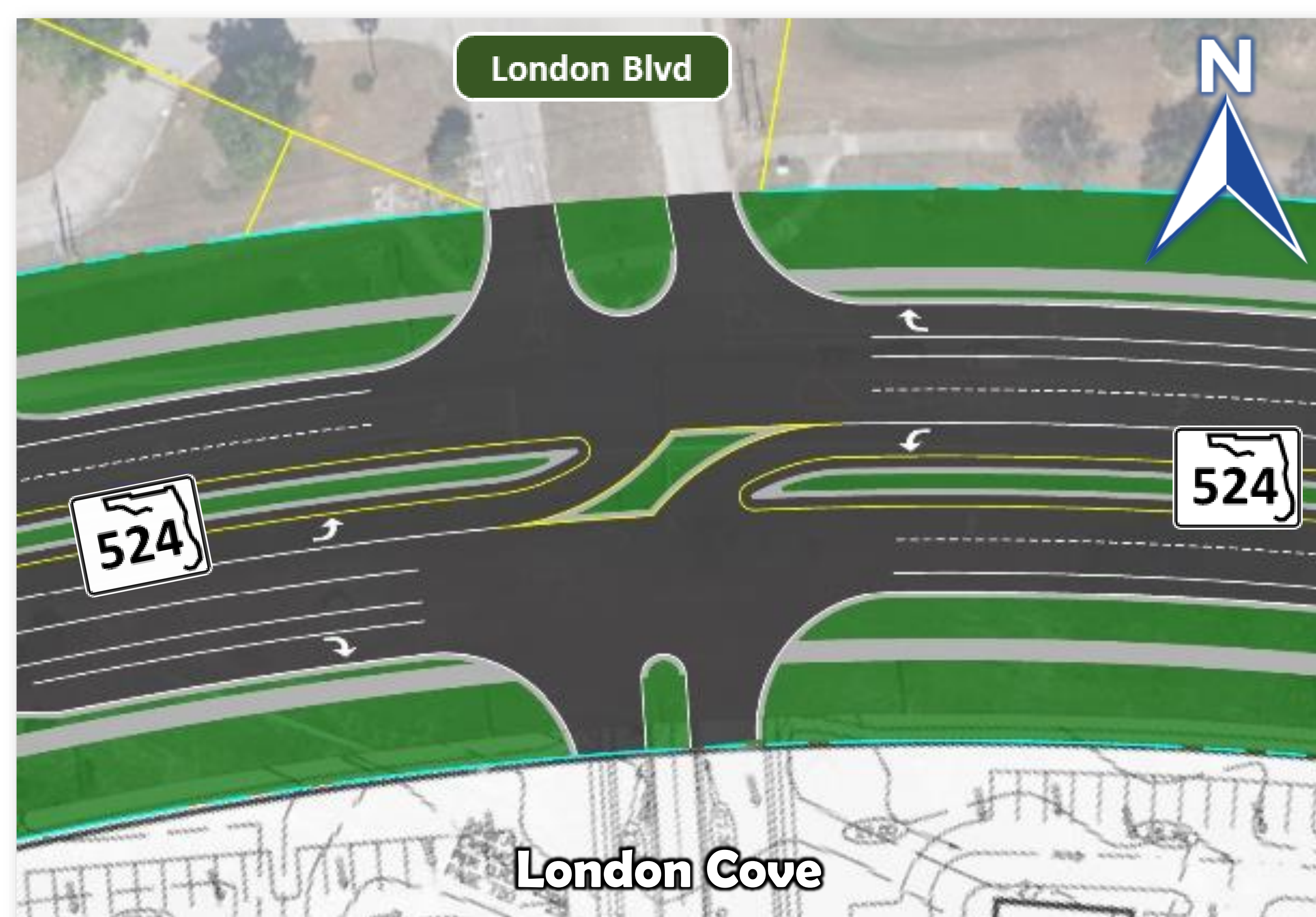
Restricted Crossing U-Turn (RCUT) Alternative
