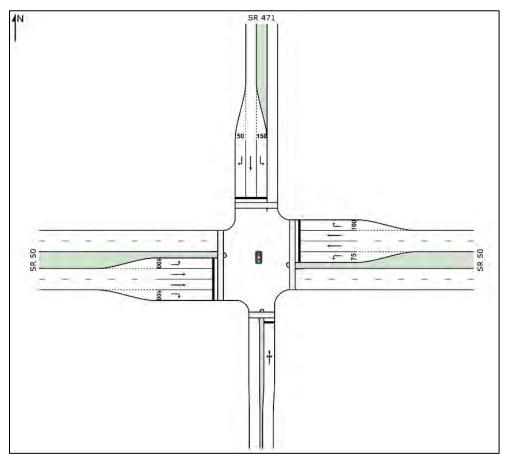
Figure 70: S.R. 50 at S.R. 471 – Signal Lane Configurations
