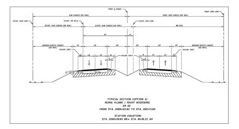
Figure 58: Rural Four-Lane Right Widening – Station 2089+02 to Station 260+71
