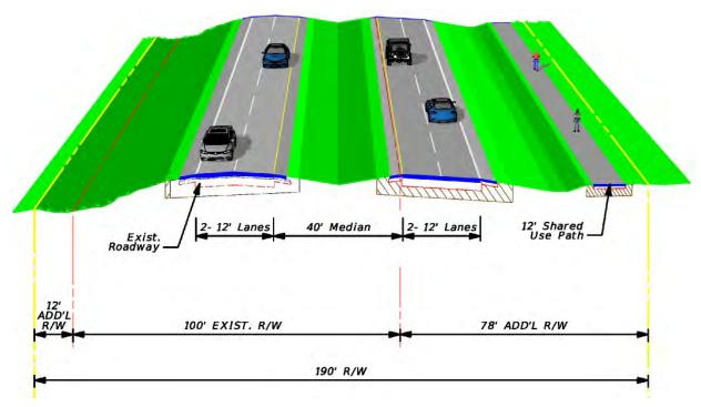
Figure 86: Typical Section – Hernando/Sumter County Line to Lee Road (Maximum ROW with New Construction and Drainage Conveyance Ditches)
