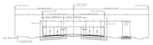
RURAL 4-LANE / TRANSITION (B) WIDENING FROM LT TO RT, RT TO LT OR CENTER WITH SHARED USE PATH / RT DITCH SR 50
