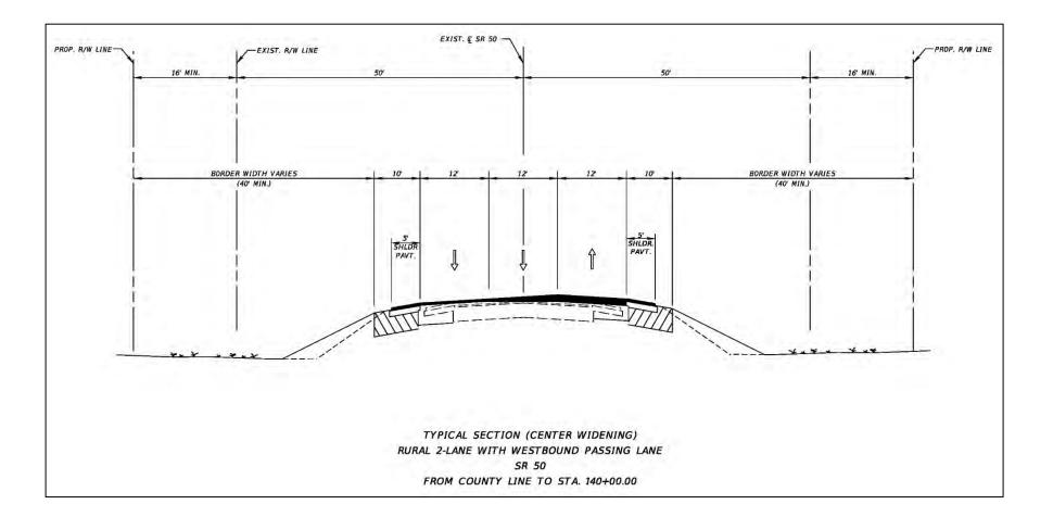
Figure 54: Westbound Passing Lane Center Widening – Station 2089+02 to Station 140+00
