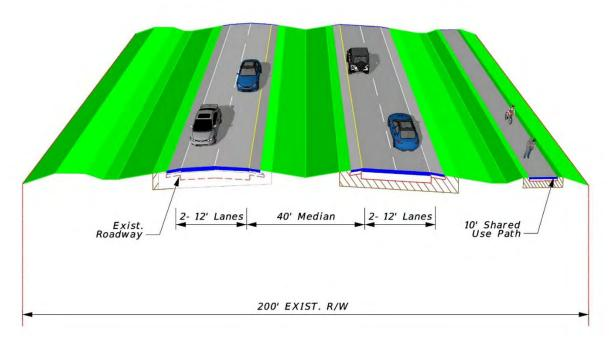
Figure 2: Typical Section – U.S. 301 to Hernando/Sumter County Line (Minimum ROW)
