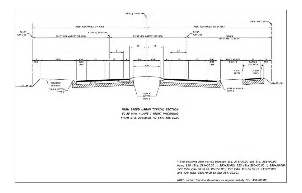
Figure 64: High Speed Urban Four-Lane Right Widening – Station 20+00 to Station 451+00
