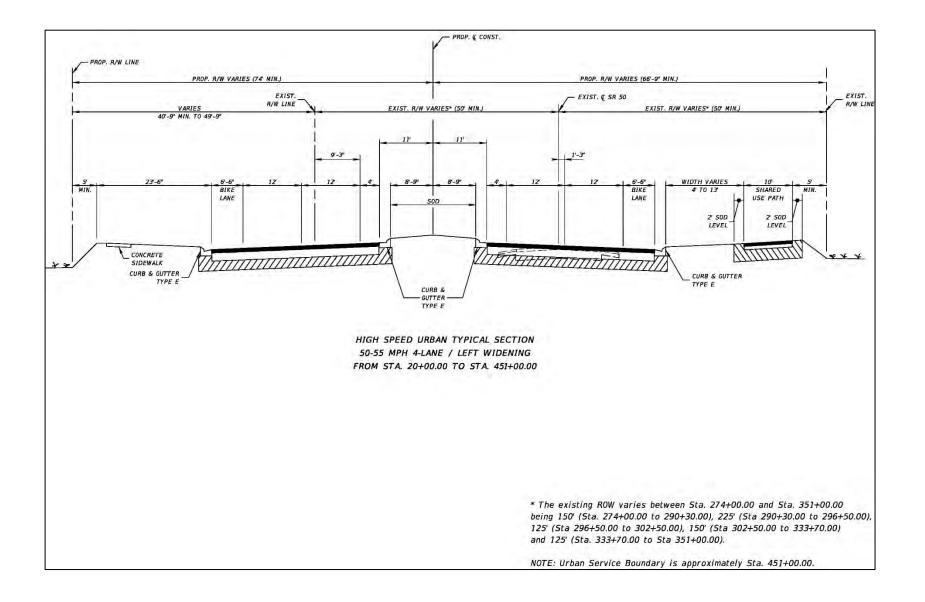
Figure 62: High Speed Urban Four-Lane Left Widening – Station 20+00 to Station 451+00
