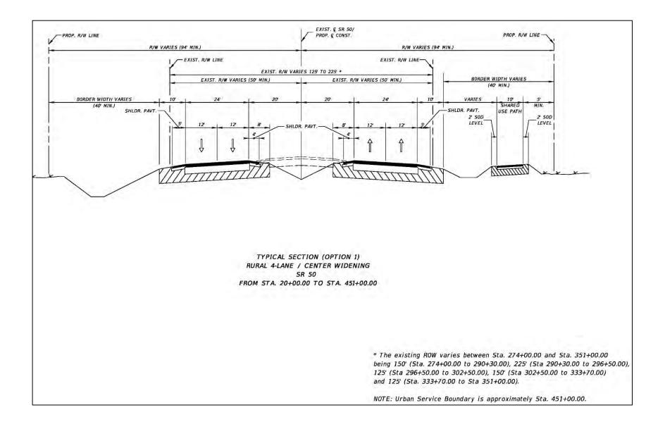
Figure 60: Rural Four-Lane Center Widening – Station 20+00 to Station 451+00
