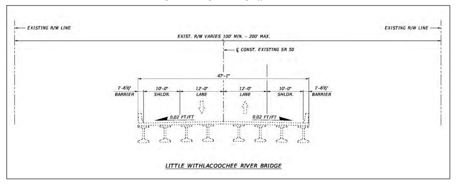
Figure 16: Existing S.R. 50 Bridge Typical Section
