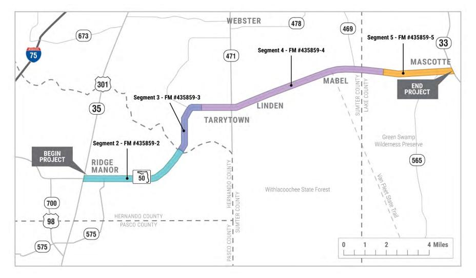
Figure 44: S.R. 50 Construction Segmentation
