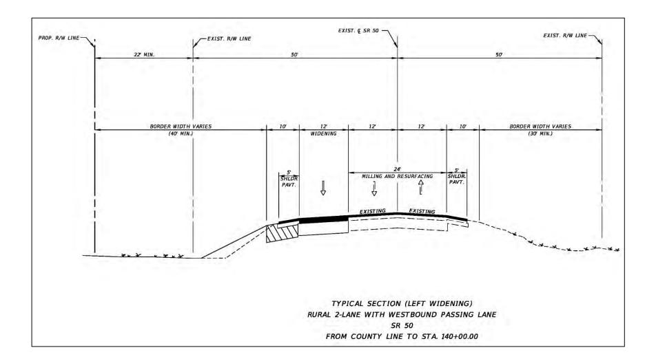
Figure 53: Westbound Passing Lane Left Widening – Station 2089+02 to Station 140+00
