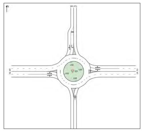
Figure 71: S.R. 50 at S.R. 471 – Multilane Roundabout Configuration
