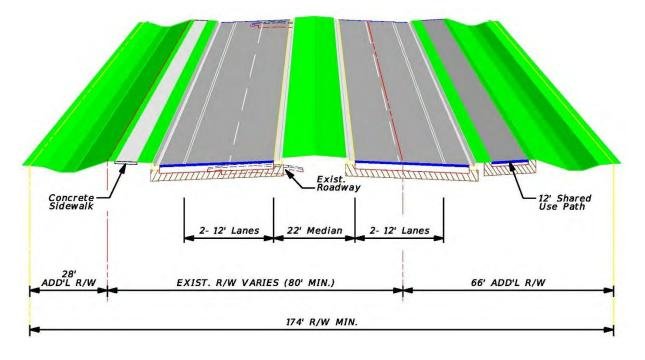
Figure 9: Typical Section – Lee Road to West of Barry Avenue (Maximum ROW with Drainage Conveyance Ditches)
