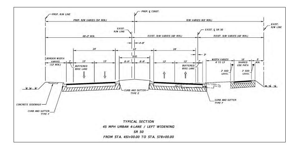
Figure 65: Urban Four-Lane Left Widening – Station 451+00 to Station 578+00
