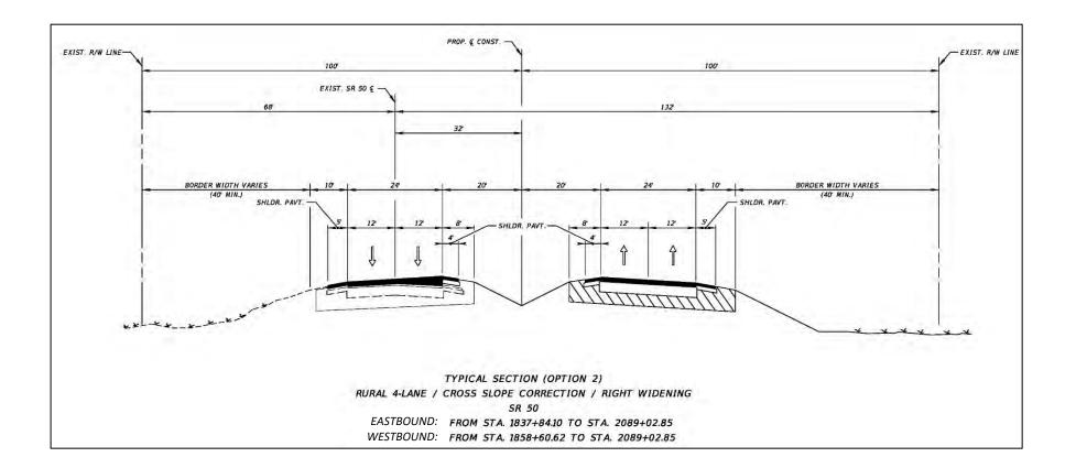
Figure 52: Rural Four-Lane Typical Section – Station 1837+84 Station 2089+02
