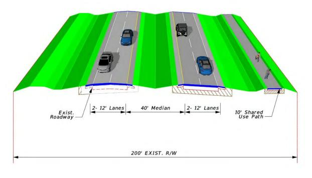
Figure 82: Typical Section – U.S. 301 to Hernando/Sumter County Line (Minimum ROW)
