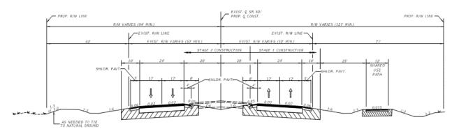
RURAL 4-LANE / TRANSITION (A) WIDENING FROM LT TO RT, RT TO LT OR CENTER WITH SHARED USE PATH / RT DITCH SR 50
