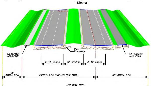
Figure 89: Typical Section – Lee Road to West of Barry Avenue (Maximum ROW with Drainage Conveyance
