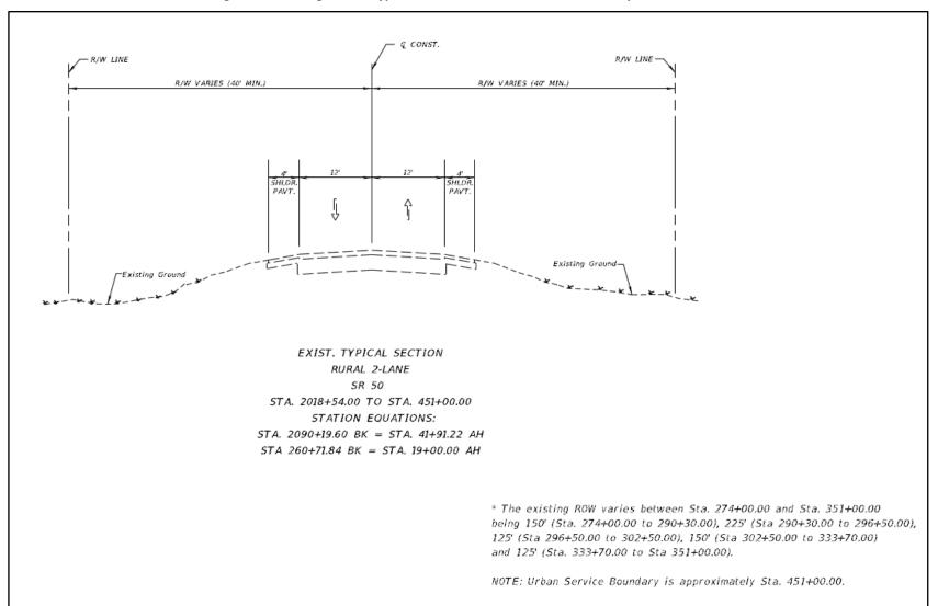
Figure 14: Existing S.R. 50 Typical Section – Hernando/Sumter County Line to C.R. 33
