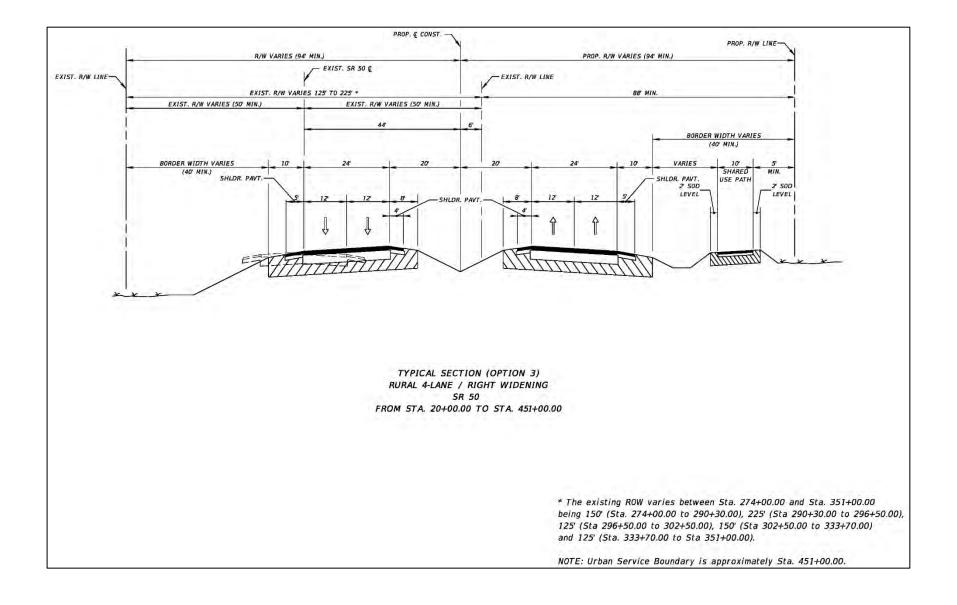
Figure 61: Rural Four-Lane Right Widening – Station 20+00 to Station 451+00
