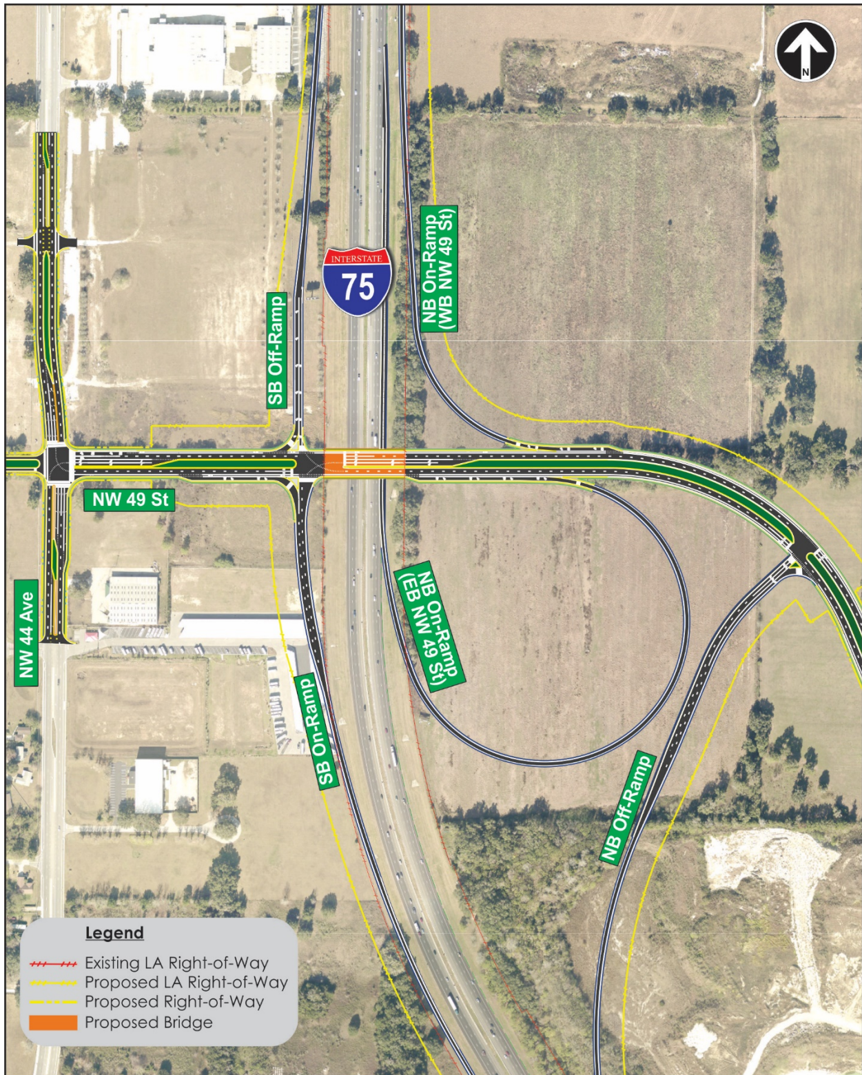
Figure 4-7 - Preliminary Parco SE Interchange
