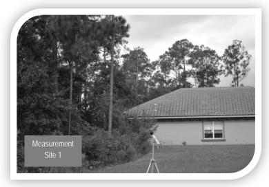
The weather during the September 10, 2012 monitoring session was 81°, and cloudy with a slight breeze. Rain was imminent. Field measurements were taken at three locations along the corridor. Measurement Site #1 is located in the II Villaggio subdivision. The meter was placed in an adjacent lot fronting SR 40, 119 feet from the SR 40 westbound travel lane, a distance that is representative of the adjacent residence shown in the photo (left). In front of the sound level meter is a stand
