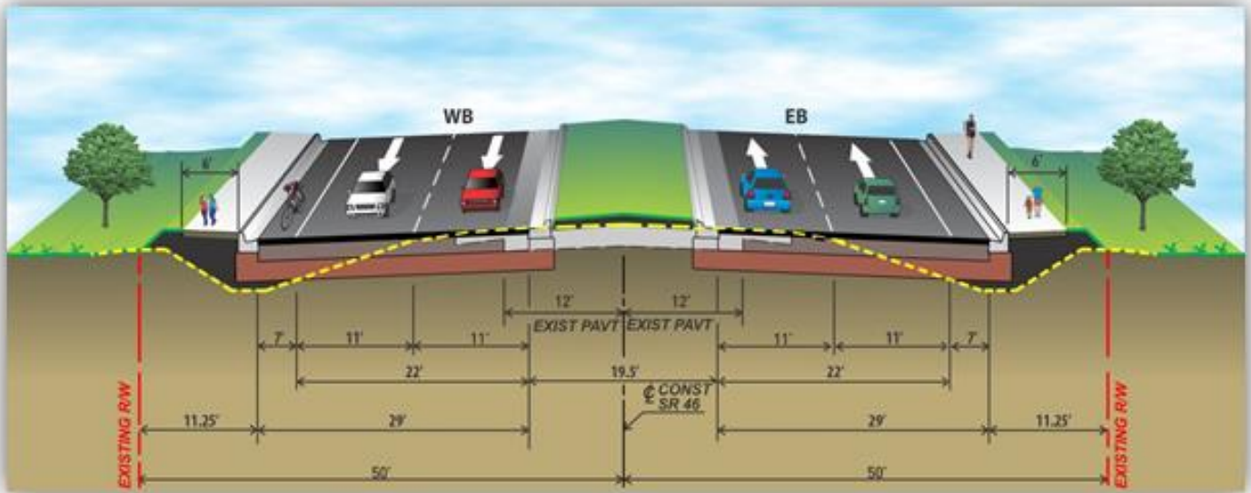
Figure 1.7 - Urban Typical Section (Centered Widening)
