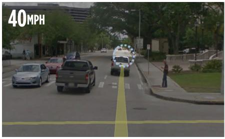
Example of driver's cone of vision based on speed.
