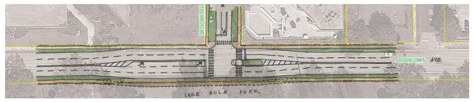
**Figure 50** | Conceptual sketch testing the feasibility of a roundabout at Broadway Avenue intersection
