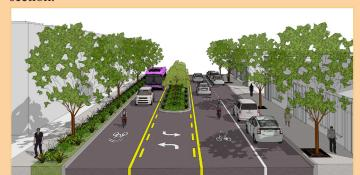
On-street parking is proposed along the south side where these are feasible based on existing driveway location and spacing.
