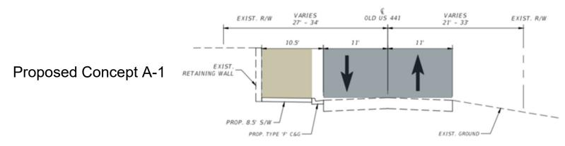
Figure 11 | Planning Concept A-1 Connector Alignment Typical Section D-D
