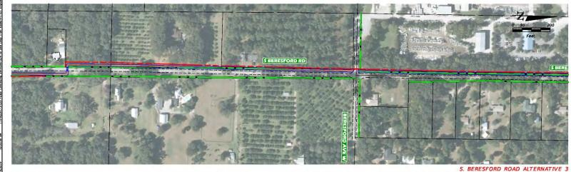
PROPERTY LINE EXISTING R/W LINE PROPOSED TRAIL PROPOSED R/W LINE PROPOSED ROADWAY RECONSTRUCTION
