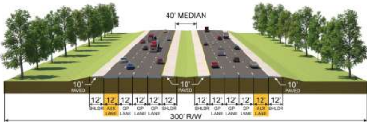
Figure 1-2 | Preferred Alternative Typical Section
