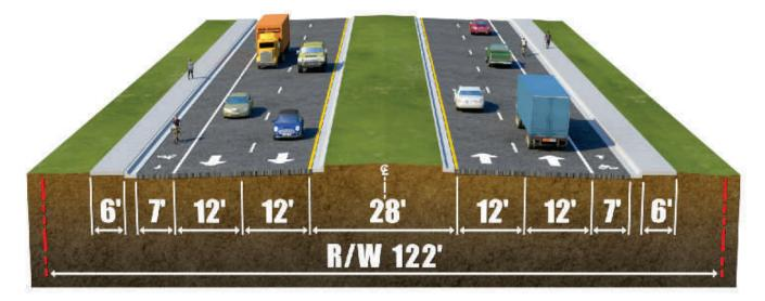
Figure 2 NW 49 Street Typical Section
